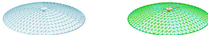
(a) Deformation status ( y=-23\text{mm} , z=-384\text{mm} ) (b) Axial forces (-981~2,532kN) Figure 16. Earthquake response of 100m lattice dome with hinge connections ( t=18.69\text{sec} , nodal load=60kN)
